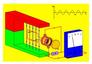
In the position shown in the diagram (left), the top and bottom parts of the loop of wire are cutting through field lines. The potential difference is shown on the voltmeter. The ends of the loop of wire are connected via slip rings and brushes to an external circuit containing a resistor (*R*). The potential difference generates a current in the circuit.
