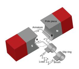
Slip rings and brushes are used to connect the rotating coil to the external circuit (see diagram). (6) "Why are they necessary?
