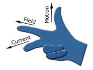
Fleming's Right Hand Rule can be applied to the section of wire at the top of the loop. Field is pointing downwards, movement is to the left, so the current direction is outwards. (try it!)
