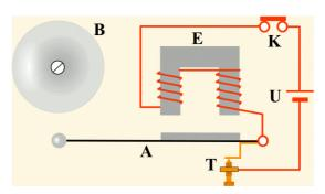
and the piece of iron is no longer attracted. The armature springs back, and the contact switch closes again. Again, a current flows and the process repeats itself. As a result, the striker repeatedly strikes the bell while switch K is pressed.
