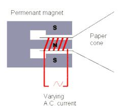
the paper cone squeeze and stretch the air producing sound waves.
