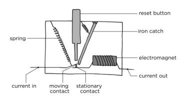
once it has blown, whereas a circuit breaker can be reset using the reset button.
