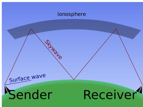
Long wave radio signals can reflect off a layer in the atmosphere called the “ionosphere”. This allows radio signals to pass around the curvature of the Earth.
