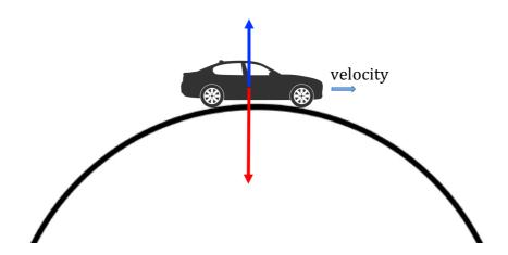
The **resultant** of the two forces acts as the **centripetal force** keeping the vehicle moving in a circle.
