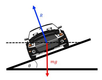
The two forces acting on the vehicle are the weight (mg) and the normal reaction (R) from the inclined track. The track is inclined at an angle  $\theta$ .
