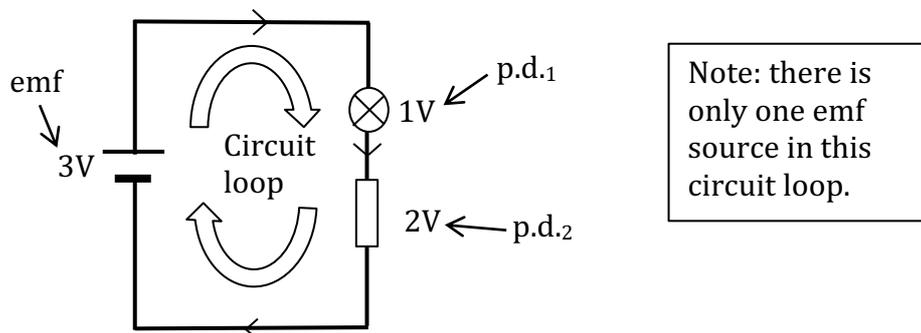
There is only one path (one circuit loop) that charges can take. Applying the rule for voltages,  $3V = 1V + 2V$ . I have chosen a 1V and 2V as the p.d.s across the lamp and the resistor. Equally, they might be 1.5V and 1.5V, or 0.5V and 2.5V (The p.d.s depend on the relative resistances of the components). What is important is that the voltage supplied by the power supply is shared out (completely) around the circuit loop.
