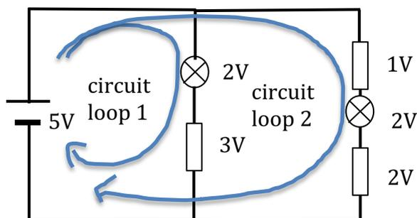
Don't worry about the individual p.d.s here. It is not important whether there is a 2V or a 1V p.d. across a particular component. What is important is that 2 circuit loops are possible and that the voltage supplied by the power supply (5V) is shared out around these 2 circuit loops. i.e.  $5V = 2V + 3V$  for circuit loop 1 and  $5V = 1V + 2V + 2V$  for circuit loop 2.
