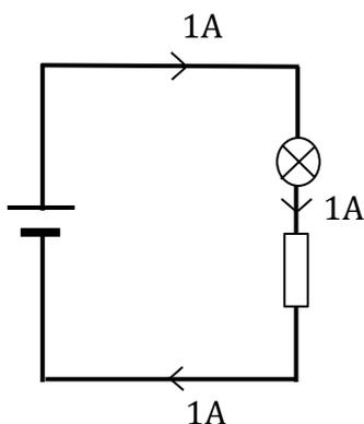
As charges can't be created or destroyed the rate of flow of charge (current) is the same at any point around the circuit - in this case 1A.
