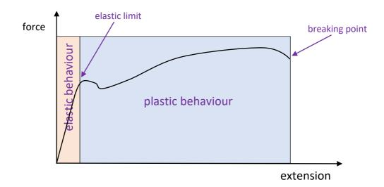
To start with the metal will stretch in a linear way. The extension is proportional to the applied force. Below the elastic limit, the metal is not permanently deformed, and will return to its original length once the force is removed.
