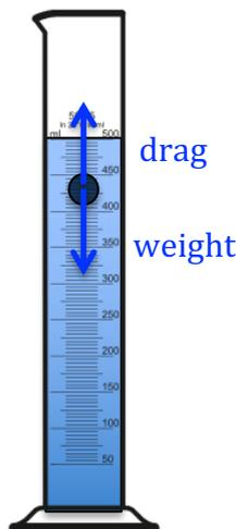
For example, we can drop a ball bearing in a measuring cylinder filled with oil and record its descent with a video recorder. If we look at the displacement at equal time intervals, we find that it remains constant. Therefore, the ball bearing is falling with a constant speed – terminal velocity.
