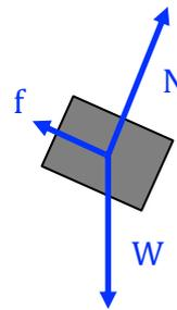
In this case we have a block on an inclined surface. On the right hand side, we have the free body diagram of the block, with only the block drawn and the external forces acting on it. In this case the forces are  $W$ =weight,  $N$ =normal reaction (reaction force from the inclined plane), and  $f$ =friction. If we found that these 3 forces add together to produce no resultant force then the block must either be at rest or moving with a constant velocity (from Newton's 1<sup>st</sup> law).
