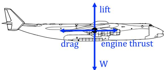
Note the specialist names for forces – 'lift' is the upward force from an aeroplane wing, 'drag' is the resistive force on an object moving through a fluid (in this case air).
