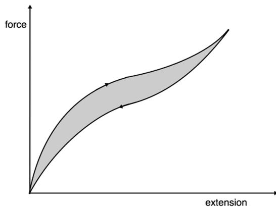
When the rubber is stretched (loading) it extends differently to when the force is removed.
