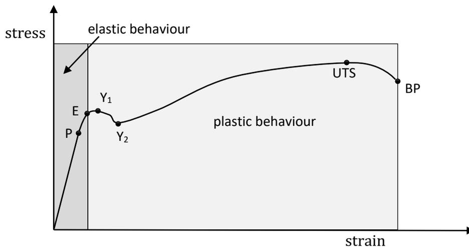
Significant points in stretching a metal:
