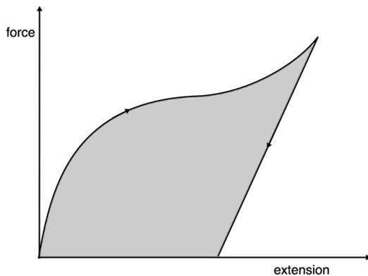
The graph on the left shows the loading and unloading of polythene. The shaded area shows the work done on the polythene during loading and the energy recovered during unloading. The shaded area shows the difference and represents the energy that has gone into the internal energy of the material, heating it and changing its structure.
