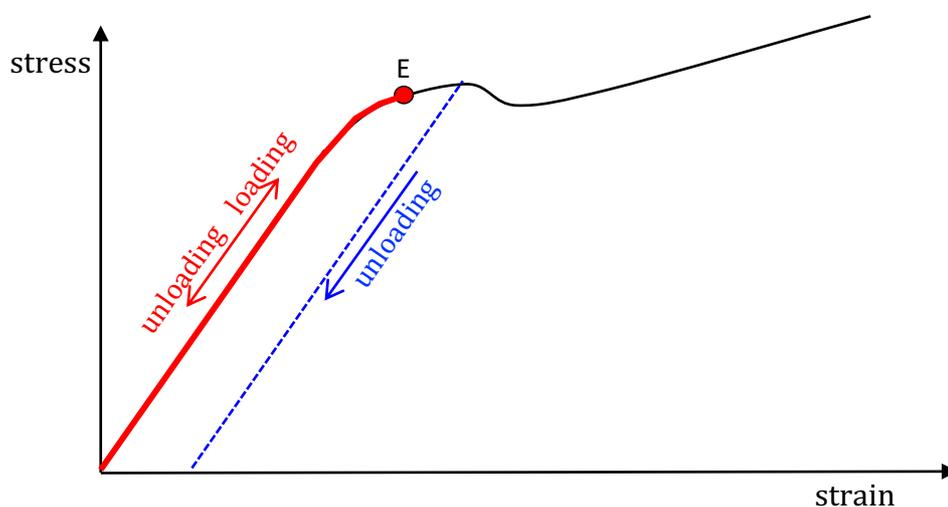
If we consider the graph, above, we can see that if we apply a stress to the material (called loading) it will return to its original shaped when we remove the stress (called unloading), providing we don't stretch it beyond E (the elastic limit). If we apply a greater stress beyond E, then the material will be permanently deformed and when the stress is removed (unloading) the material is permanently strained. This is represented in the diagram by the dashed line.
