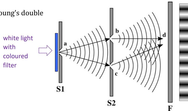
White light is passed through a coloured filter. The filtered light is of one frequency. Next, the light passes through one slit. Because we effectively have a point source of light, photons arriving at the double slit will have a constant phase difference (in this case, zero) determined by the path difference between the single slit and the two slits. In this case the path lengths are the same.
