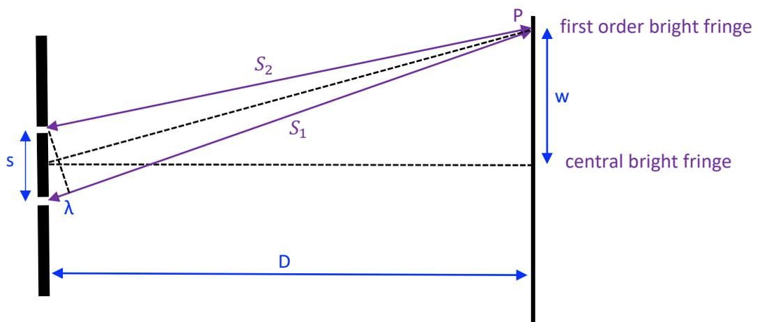
Where  $s$  = slit separation,  $D$  = slit to screen distance,  $w$  = separation of high intensity (bright fringe) on the screen,  $\lambda$  = wavelength of light,  $S_1$  and  $S_2$  are path lengths from slits to screen.
