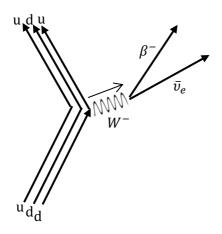
A down quark is changing to an up quark. The other two quarks remain unchanged. The result is that the neutron (*udd*) changes to a proton (*uud*).
