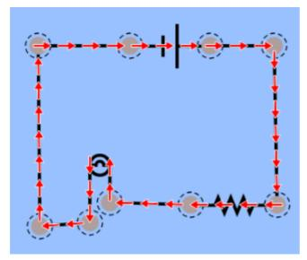
This is a series circuit consisting of a cell, a resistor and a light bulb. The arrows show the direction of the flow of 'conventional' current. Remember, by convention, that current is the 'rate of flow of <u>positive</u> charge', and so flows from the positive terminal of the cell around to the negative terminal.
